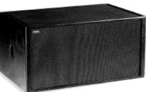
The **G-118S** is a symmetrical double loaded compression system of fourth order with twin chambers. The rear load being closed and the front one being tuned to 65 Hz and loaded with an exponential horn at the mouth of the resonator.
