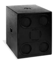
The **SG-118** unit is a subwoofer system of double symmetrical load of sixth order, with independent tuning in each chamber. The rear load of the loudspeaker is tuned to 35 Hertz and the frontal load to 80 Hz. We achieve an effective sub-bass response with a relatively small enclosure.
