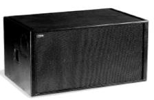
The unit **TSG** is a symmetrical double loaded compression system of fourth order with twin chambers. The rear load being closed and the front one being tuned to 65 Hz and loaded with an exponential horn at the mouth of the resonator.
